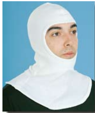
NK 2310 CA Sock Hood (full face) HAZARD RISK CATEGORY 2 • ARC RATING 9.4 cal/cm 2 • 2-ply stretch white NOMEX® with 2-ply cape • Flame resistant and launderable STOCK
