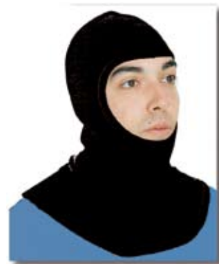
CXK 2310 Sock Hood (full face) HAZARD RISK CATEGORY 2 • ARC RATING 23 cal/cm 2 head area • ARC RATING 12 cal/cm 2 neck area • 2-ply stretch 7.4 oz. Knit CarbonX® with 1-ply cape • Flame resistant and launderable STOCK
